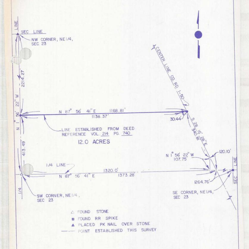
I hereby certify that I have surveyed the premises and prepared the above plat and that said at is correct to the best of my knowledge and belief. All dimensions are shown in feet and decimal parts thereof. This survey has recorded in vol. 100 Page 107 of the Williams County Record of Surveys.
